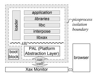
Figure 1: The Xax architecture. Everything inside the picoprocess ( $\S3.1$ ) isolation boundary is untrusted. The Xax Monitor mediates access to the outside world, employing existing browser mechanisms ( $\S3.3$ ) to implement xaxcalls from the picoprocess. The PAL ( $\S3.2$ ) provides a consistent Application Binary Interface (ABI) across OS platforms. Above the ABI, the specific structure can vary; the depicted structure is one we have found useful when porting code ( $\S3.4$ ).
