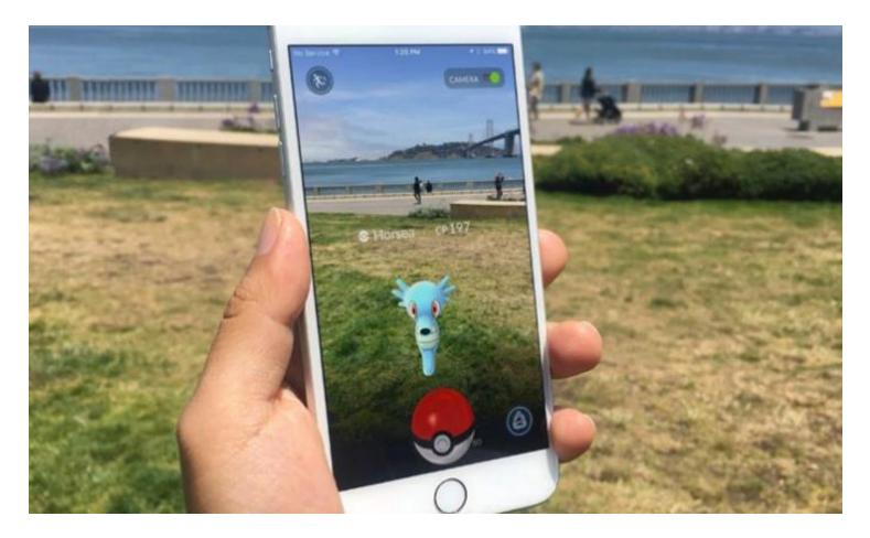
• Handheld AR, touch input, GPS/compass sensors
