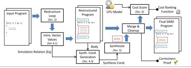
Figure 4. Overview of the auto-vectorization algorithm.
