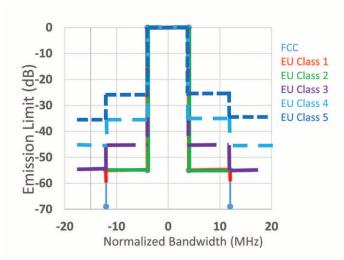
FIGURE 5. Spectrum masks (scaled) for FCC and ETSI Class 1 through Class 5.
