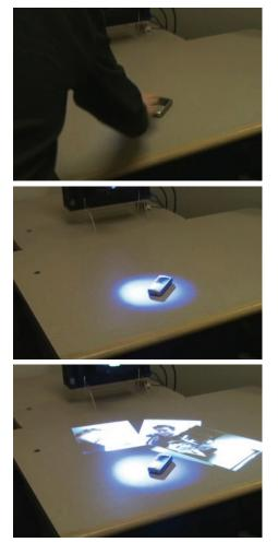
Figure 7. BlueTable prototype connects automatically to cameraphone via Bluetooth, transfers photos, and spills them onto interactive surface.
