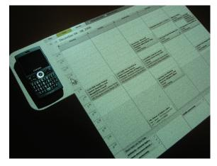
Figure 10. Mockup of a complex user interface (calendar application) that spills out of a mobile device onto BlueTable.
