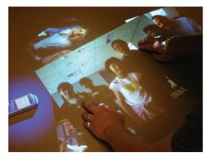
Figure 8. Photos may be scaled, rotated and moved on the desk by using one or both hands. Optical flow techniques are used to recover the motion of the hands. This motion is then modeled as a combination of simultaneous rotation, scaling and translation movements. An individual photo is brought to the top of the stack of multiple photos by touching any part of the photo with an outstretched finger.
