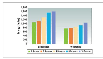
Figure 5. Energy used when storing to local flash memory vs. using WearDrive, based on between 1 and 16 sensors generating data continuously at 1 Hz for 24 hours. A typical smartwatch battery stores between 3000—6000 Joules of energy.
