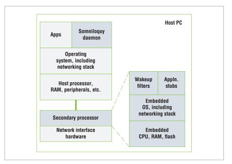
Figure 3. New components, shown in blue, must be added to a mobile device to implement Somniloquy. In addition to the low-power secondary processor and associated embedded operating system, wakeup filters and application stubs interact with the main processor via a Somniloquy daemon.
