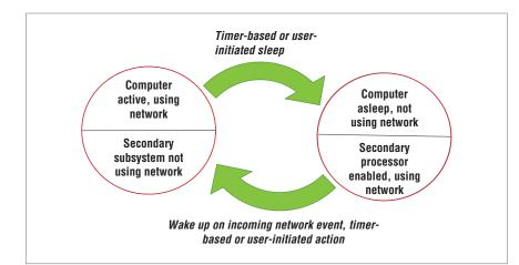
Figure 1. Somniloquy has two main operating states—in one, the main CPU is active; in the second, control resides with the secondary processor while the main CPU sleeps. The transitions between them are initiated by the events shown in the figure.
