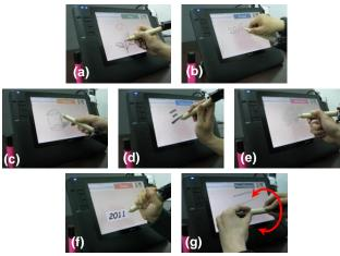
Figure 2. Virtual implements. (a) Pen (b) Eraser (c) Sketching pencil (d) Chinese calligraphy brush (e) Airbrush (f) Stamp (g) Pencil sharpener for width adjustment.
