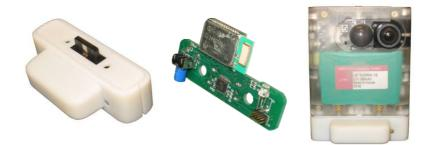
**Fig. 6.** The Bluetooth expansion adapter and the PCB shown on the left, and the assembled unit shown attached to a SenseCam on the right. It plugs directly into the SenseCam expansion connector and is secured from below with two M3 screws.
