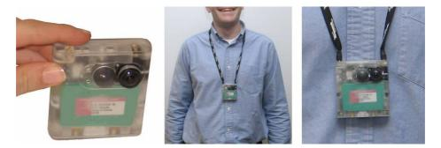
**Fig. 1.** The SenseCam v2.3 prototype shown standalone and as typically worn by a user. The model pictured here has a clear plastic case which reveals some of the internal components.
