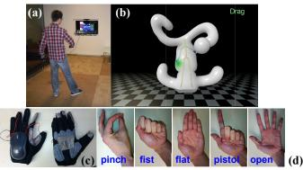
Figure 4. (a) BodyAvatar setup. (b) Software interface. (c) Gesture gloves. (d) Hand poses (shown without glove for clarity).
