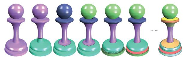
Fig. 3. Illustration of the segmentation process. The segmentation is initialized with 1 proxy (leftmost), new proxies are progressively inserted. From left to right, 1–6 proxies and final result with 13 proxies (rightmost).
