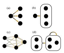
The simplest Fig. 3. Matching Neighbors compression allows for leaves of "star graphs" (a) to be collapsed into a module (b). A simple extended matching allows for cliques as in (c) to also be grouped (d). In (d) the edges in the clique module are removed and implied by a self-loop: an arrow from the module to itself.
