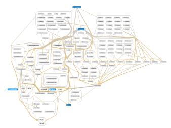
(b) A compressed version (using the heuristic described in §3.3) has 17 modules, reducing the visible edge count to 208. Obviously, at this scale individual edges are difficult to follow, yet the groupings are also interesting since they show the members that are accessed together.
