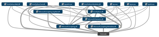
(a) The top-level component graph produced by the Visual Studio code-dependency analysis tool for the IronPython code base with 39 edges.
