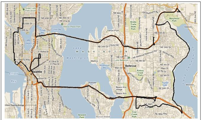
Figure 2: This is the GPS data we used for testing in the Seattle, Washington, USA area. The trip starts in the upper right near Marymoor Park. It consists of 7531 GPS points sampled at 1 Hz, and it covers about 80 kilometers (50 miles) over about 2 hours.
