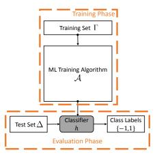
Figure 1: A two-stage design flow of a machine learning task: training phase in which the ML algorithm  $\mathcal{A}$  is applied to training set  $\Gamma$  to learn classifier h, and evaluation phase to judge the quality of h on test set  $\Delta$ .
