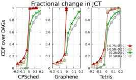
Figure 17: Fractional change in the job completion time (JCT) of DAGs with various schedulers when task durations and resource profiles are mis-estimated.
