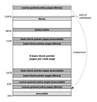
Figure 3: The user-level address space layout in GRIFFIN.
