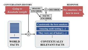
Figure 3: Knowledge-grounded model architecture.
