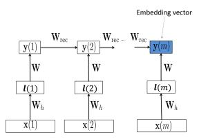
Fig. 1. The basic architecture of the RNN for sentence embedding, where temporal recurrence is used to model the contextual information across words in the text string. The hidden activation vector corresponding to the last word is the sentence embedding vector (blue).
