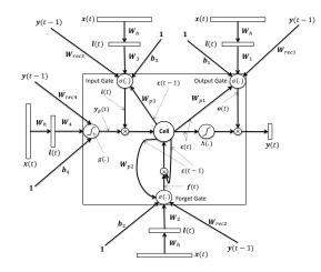
Fig. 2. The basic LSTM architecture used for sentence embedding
