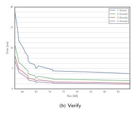
Figure 2: Runtime of the parallelized version of Sign and Verify of Fish using an increasing number of threads. The x-axis shows the running time, while y-axis shows the various LowMC parameter sets, sorted by signature size (as in Figure 1).
