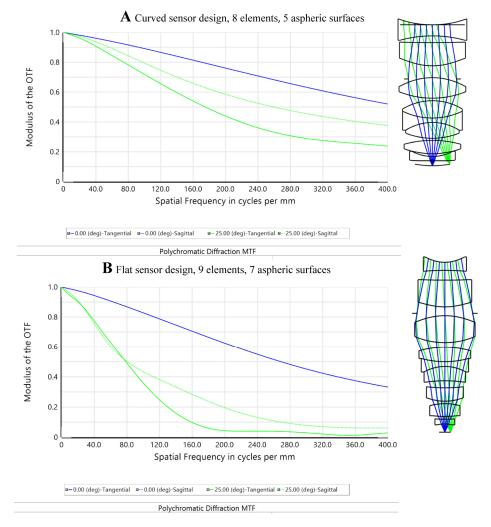
Fig. 7. As-designed MTF for curved vs. flat designs for f/1.2, 1/2.3" CMOS sensor with 50 ° field of view. A) Curved sensor, optimized for an 18.74 mm radius of curvature sensor. B) Flat sensor optimized design. The curved system has almost double the sharpness at every field angle, despite having 1 less element and 2 fewer aspherical surfaces. The flat sensor design is also much larger.
