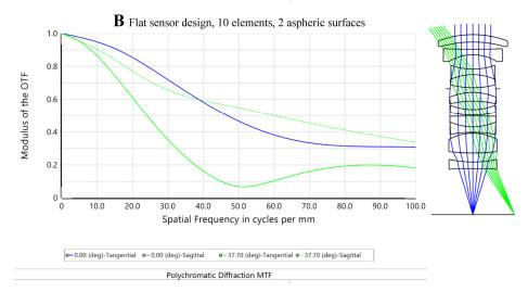
Fig. 10. Design study comparison between the curved sensor optical system A) and flat sensor B). 28 mm focal length, f/1.7, 75° diagonal field of view, 43 mm image circle. Flat lens B) has 10 elements and 2 aspherical surfaces. Curved sensor lens A) has seven elements and one aspherical surface. At MTF50 the curved sensor design A) has 1.3x the spatial frequency response of the flat design B) despite having fewer elements.
