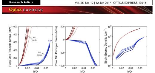
Fig. 3. Finite element predictions for the peak stresses and volumetric strain energy density developed as a function of normalized center displacement for the fixed perimeter and free edge molding operations for thicknesses ranging from 40  $\mu$ m to 100  $\mu$ m and a die size of 22.3 mm x 28 mm.
