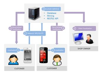
Figure 1: Architecture of the Location-log system
