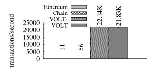
FIGURE 7—Transaction processing throughput of VOLT and its baselines (§6.1) for our payment network application (§5). VOLT does not rely on mining, so its throughput is orders of magnitude higher than Ethereum. We find Chain to be unoptimized for throughput, but we include it here for rough comparison. Both VOLT and VOLT- achieve excellent throughput due to their powerful BSP. See text for additional details of the experiment.
