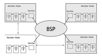
FIGURE 1—High level architecture of VOLT. Members run a simple verifier process that communicates with the BSP, executes local end-to-end checks, and outputs a consistent view of the BSP's ledger. The internal implementation details of the BSP and other member nodes (denoted with shaded color) do not compromise the safety guarantees that VOLT's verifier ensures to a correct member (denoted without a shaded color). Dotted arrows represent optional communication channels.
