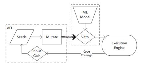
Fig. 3. The veto model used by Augmented-AFL. Mutations which target no useful locations are not executed.
