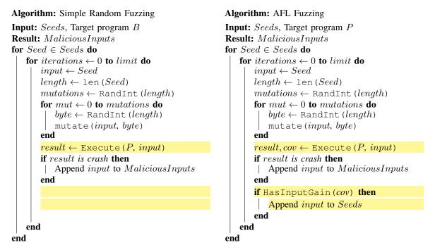
Fig. 1. Comparison of the AFL fuzzing algorithm with a simple random fuzzing algorithm. The *mutate* function mutates a byte of the input in place using various techniques such as bit flips, bit rotations or arithmetic operations. The *Execute* function executes the target program with the mutated input and reports on crashes. For AFL, the Execute function also reports the induced code coverage (*cov*).
