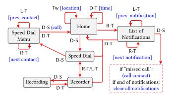
Figure 6: State machine for the app on smartphone. During state transitions, the app explicitly reads out the text corresponding to the item within square brackets.
