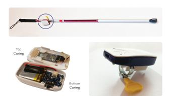
Figure 1: GesturePod. Top image shows the pod attached to a white cane. Bottom left image shows the interior of the pod.
