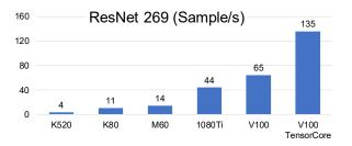
Figure 1: Single-GPU training throughput for ResNet 269 measured with MXNet on EC2 g2, p2, g3 and p3 instances, and a local GTX 1080 Ti machine, while maximizing GPU memory utilization. Per chip GPU throughput on ResNet 269 in the cloud has increased 35x since 2012.
