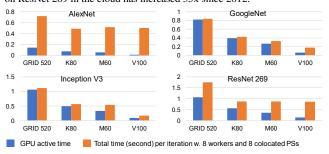
Figure 2: The overhead of distributed training gets larger as GPUs get faster. The framework can no longer hide communication latency, and faster GPUs no longer improve training throughput. With today's fast GPUs, distributed cloud DNN training time is chiefly spent waiting for parameter exchanges.
