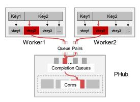
Figure 8: The process of mapping a chunk to a core in PHub using fine grained key chunking. Keys are chunked into virtual keys. The highlighted key is delivered to a highlighted (fixed) core through a highlighted (fixed) queue pair and completion queue.
