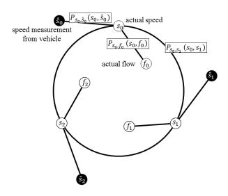
Figure 3: This is a graphical representation of the variables for a road network with three measurement stations. The measured variables are associated with the filled-in circles, and the unknowns are in the white circles. Each edge is represented by a joint PDF.
