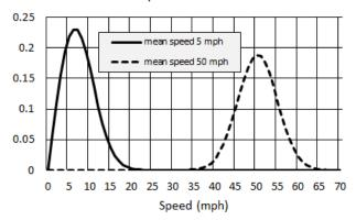
Figure 4: These are two Rician speed distributions  $P_{s_i}(s_i)$ , assuming GPS precision of  $\sigma_g = 3$  meters and a GPS sampling interval of  $\Delta t_i = 2$  seconds.
