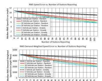
Figure 10: The solid lines show how the speed error (top plot) and demand-weighted speed error (bottom plot) change with the number of randomly-ordered stations reporting and the number of vehicles reporting from each station. The corresponding dashed lines show the corresponding errors when the stations report in descending order of estimated VOI. The dashed lines always show lower error than their solid counterparts, meaning the VOI method gives consistently lower error.
