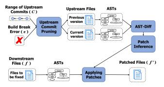
Figure 10: Overview of the automated patching.
