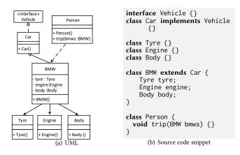
Figure 1: UML class diagram example
