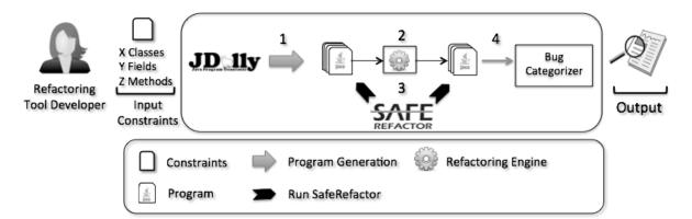
Fig. 1: A technique for testing refactoring engines.
