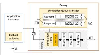
Fig. 4: BumbleBee extends the Envoy sidecar (BumbleBee components marked as yellow).
