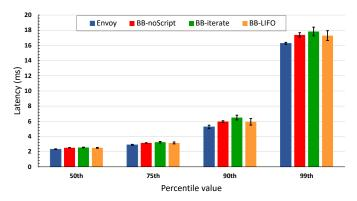
Fig. 16: Micro-benchmarks with wrk2 show that BumbleBee adds no additional overhead compared to Envoy up the 99th percentile. However, the additional cost of iterating over a message queue becomes apparent at the very tail of distribution.
