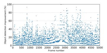
Fig. 8: BumbleBee enables the traffic-monitoring application to send 360p frames when possible and avoid head-of-line-blocking by selectively downsampling frames to 180p. Each blue data point represents the percentage of additional objects that the BumbleBee-enabled application detects in a frame compared to sending all 180p frames. The 3444 frames (out of 5000) are downsampled to avoid exponential queuing delays. These frames gain zero percent improvement.
