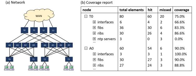
Figure 5: Example coverage report (b) for a datacenter network (a) generated from evaluating the BGP network reachability test from §5 against the datacenter network.
